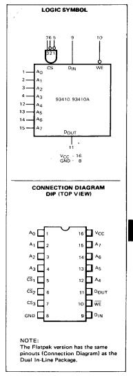
FUNCTIONAL DESCRIPTION - The 93410/93410A are fully decoded 256-bit Random Access Memories organized 256 words by one bit. Word selection is achieved by means of an 8-bit address, An through A7.
